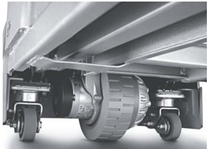
Optimum traction and castor wheels for perfect stability 3
